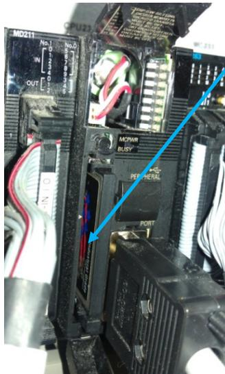
Insert the CF Memory card into the slot with the label to the left.
